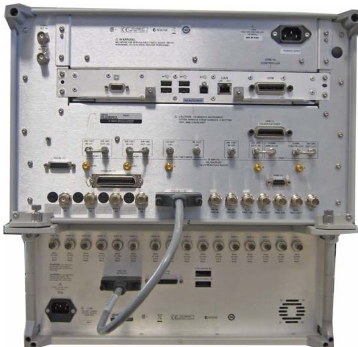
Figure 30 N5242A Test Set I/O Cable Connection
